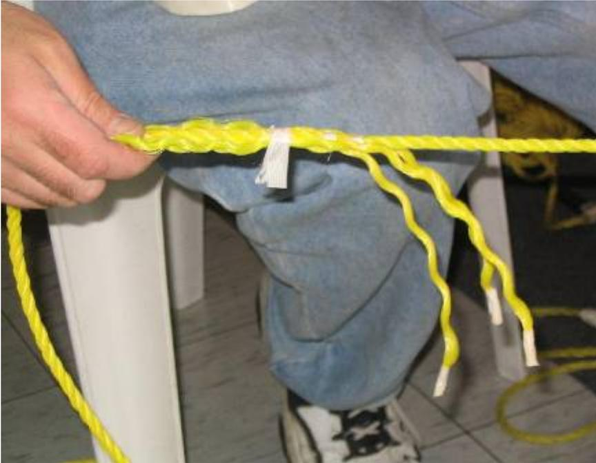
**Figure 13 – Tape One Side of Splice**
