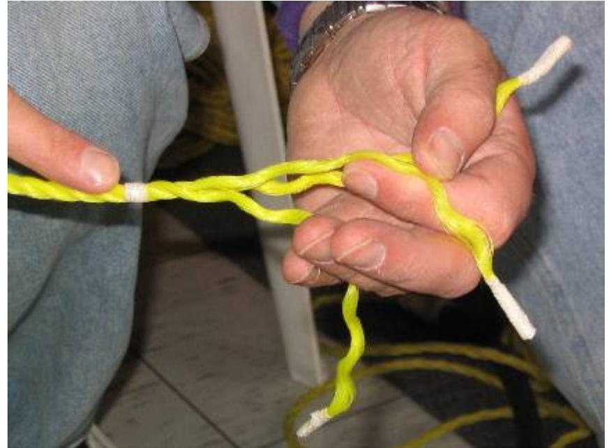
Figure 10 – Wrap of Tape on Ends to Eliminate Destraining
