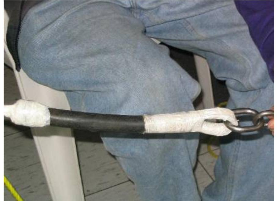
**Figure 8 – Completed Glider End of Tow Rope**
