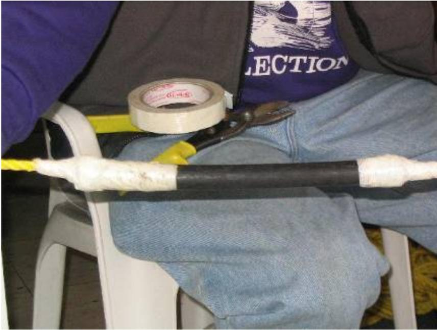
**Figure 17 – Completed Weak Link Splice**
