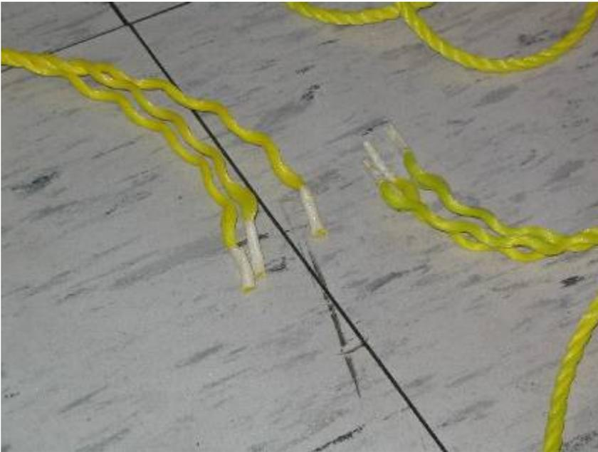
Figure 9 – Ends of Weak Link and Tow Rope Prepared for Splice
