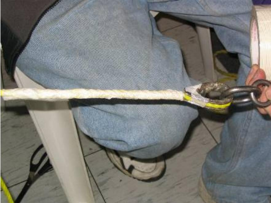
**Figure 7 – Taped Splice**
