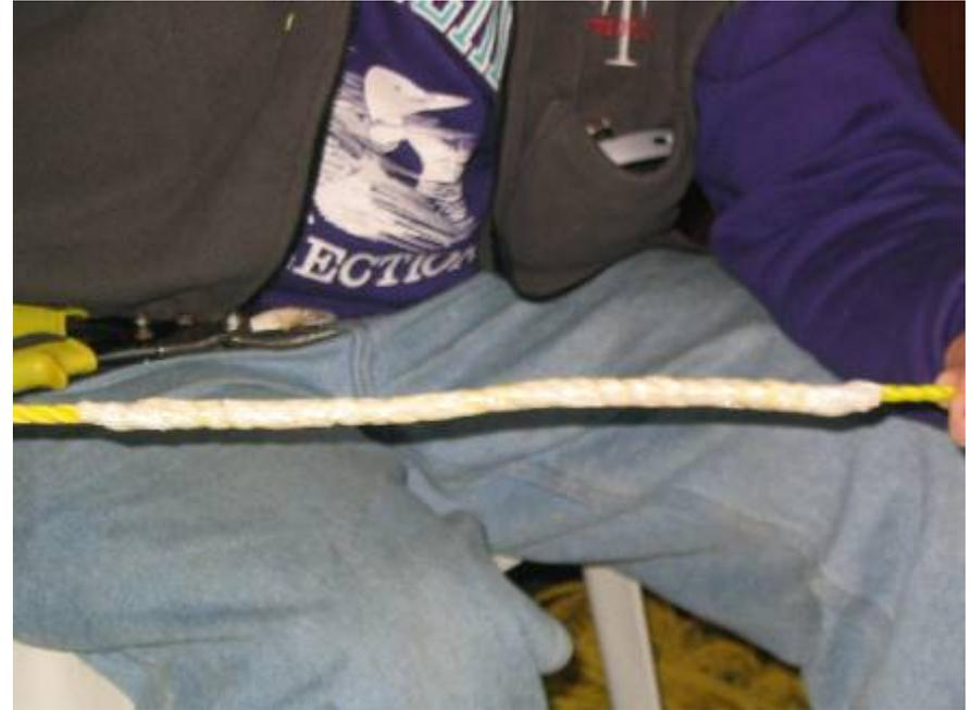
Figure 16 – Taped Splice
