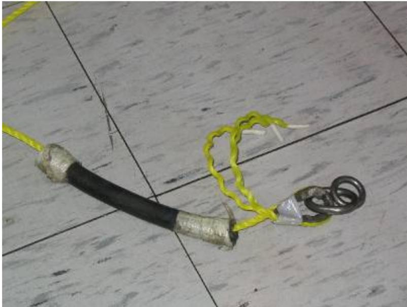
**Figure 4 – Create Weak Link & Terminate Glider End**
