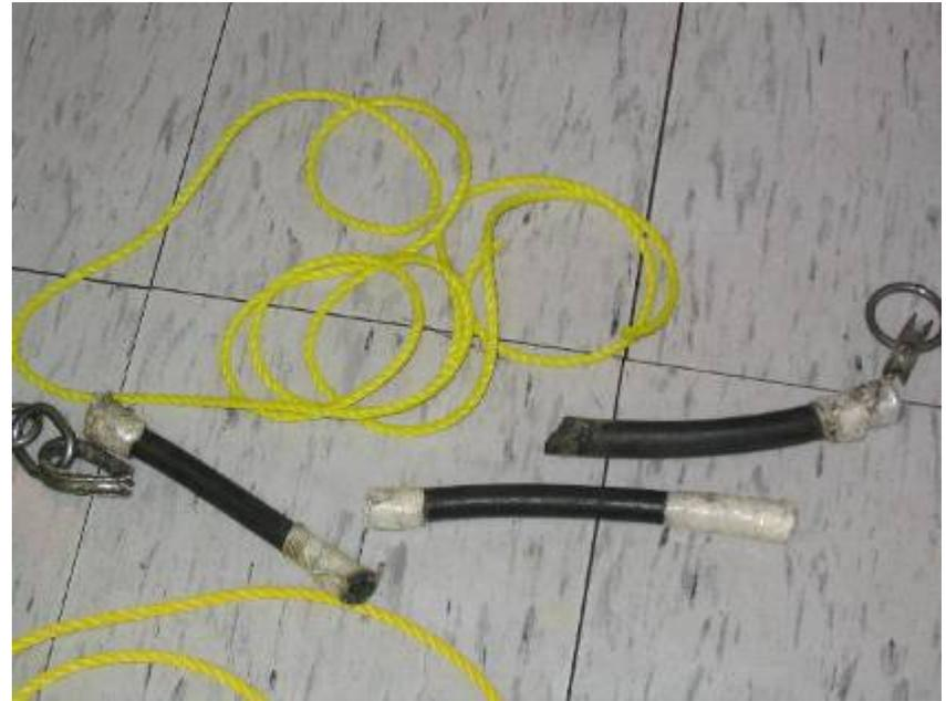
**Figure 3 - Prepare Weak Link and Glider End**
