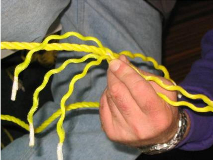
**Figure 11 – Mated Rope Showing Strands Emerging Alternately from Each Rope**
