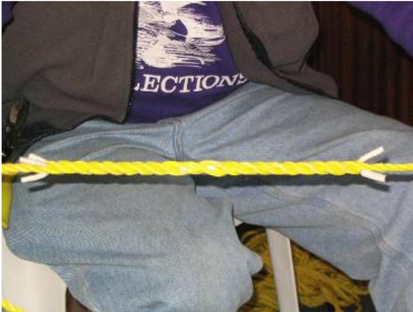
Figure 15 – Completed Splice - Notice Smooth Regular Weave
